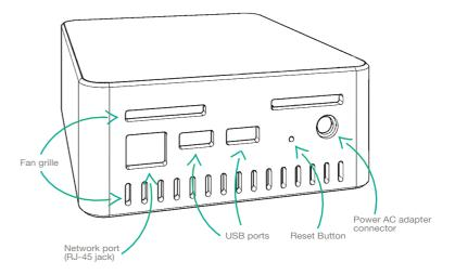
Do not block the fan grille (located on the side of the device)! If you are putting the unit on its side, make sure the side with the grille **NOTE:** is pointing up!
